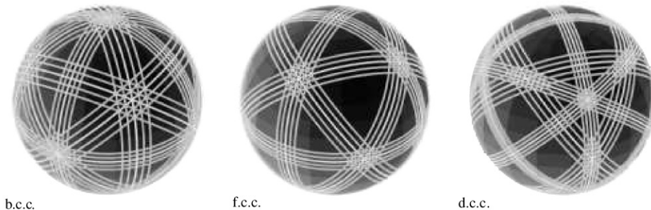
Fig. 6. Visibility maps for the two largest fringes visible from body-centered, face-centered, and diamond face-centered lattices. Sphere diameter (relative to bandwidth and fringe spacing) is proportional to specimen thickness, here chosen to be about 5 times the cubic cell side a . Note the dominance of crossed \{110\} fringes at the 3-fold \langle 111 \rangle zone in the body-centered case, the dominant crossed \{111\} fringes at the 2-fold \langle 110 \rangle zone in the face-centered cases, and the wider disparity between largest and next-to-largest spacings when the diamond glide is added to the lattice.
